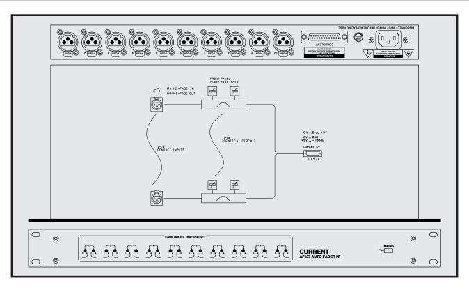
10ch automatic fader interface It is fitted by STUDER A779 console Input out individual time set 19 inches 1U size
