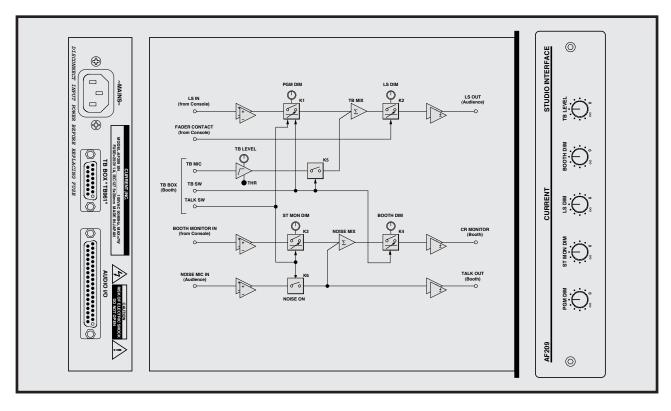
Bidirectional talkback system Each channel independent DIM level control Remote TB box It is most suitable for DJ booth 1U half rack size
