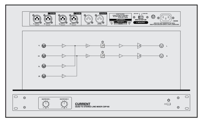
2 stereos to one Super low noise It is most suitable for 4ch microphone preamplifier All the world AC voltage support 19 inches 1U size
