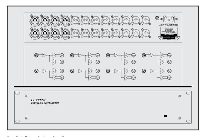
Two distributes 8 channel audios Super low noise High-quality sound Super low distortion 19 inches 2U size
