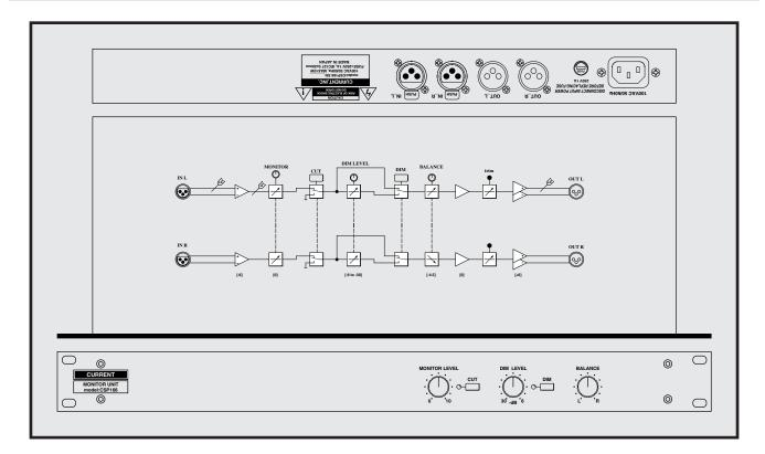
Simple monitor unit Monitor cut Variable DIM level Balance XLR input and output 19 inches 1U size
