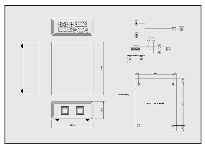
2:1 AES switcher BNC connector Locality, remote control Bypasses it with power off Compact
