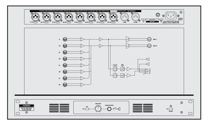
Mix in 8ch of high quality It is most suitable for monitor of DAW Monitor is possible with front panel speaker Headphone monitor is possible 19 inches 1U size
