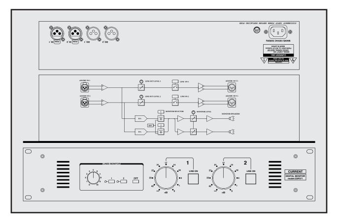
2 path digital audio level control Line ON/OFF Line out volume control Stereo monitor speaker 19 inches 2U size
