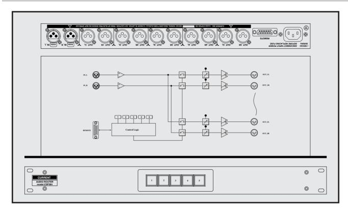
Routing to 5 routes in a stereo source XLR connector
