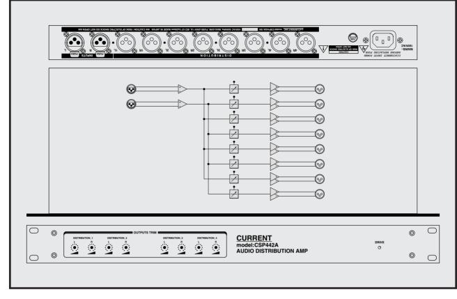
4 distributes for stereo source 8 distributes mono source Super low noise High-quality sound All outputs with trim 19 inches 1U size
