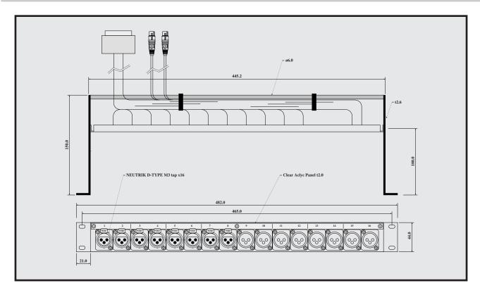
16ch connecter panel It is compatible by neutrik D-type 100mm recession setting Fixing Bar
