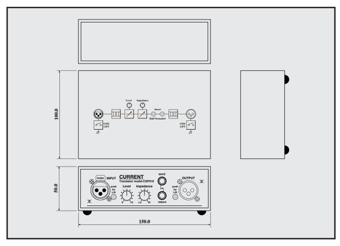
Trans box such as the Swiss Army knife It is variable in output level and impedance As XLR isolator As a re-amplifier As a direct box As a volume box As balance unbalanced conversion Jensen made transformer use Compact
