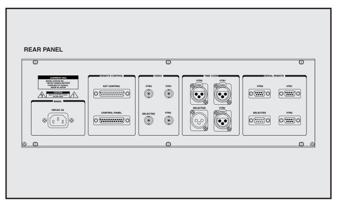
9P remote switch of 3:1 Timecode switch of 3:1 Composite video switch of 3:1 Remote control 19 inches 3U size
