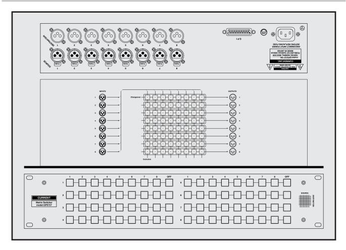
8 input, 8 output Balance input and output Exclusion function It is most suitable for the transfer of the phone line Plain interface 19 inches 2U size
