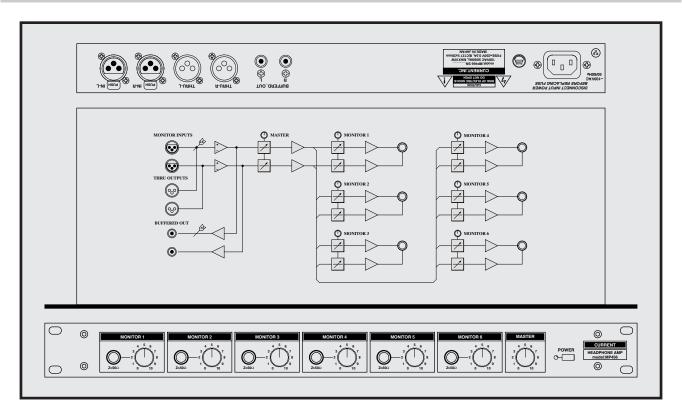
6 channel stereo headphone amplifiers XLR connecter input It is with the through output High power The master volume 19 inches 1U size
