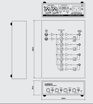
Stereo phone amplifier Balance, XLR input 4 independent output Earphone or headphone Compact and robust
