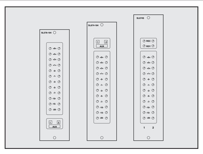
Highly visible LED from left and right Stereo VU Peak hold Various display
