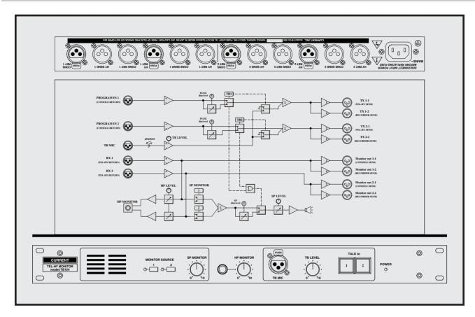
Bidirectional talkback system Speaker monitor Headphone monitor With REC out Telephone hybrid line monitor 19 inches 1U size
