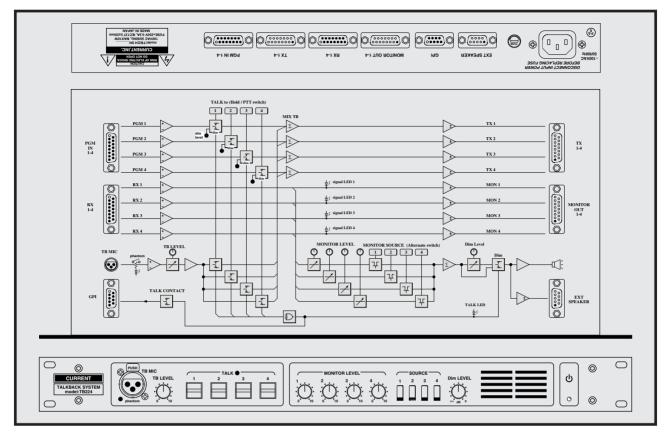
4 bidirectional talkback systems Speaker monitor RX signal indicator Variable monitor Monitor DIM level Output for external monitors 19 inches 1U size
