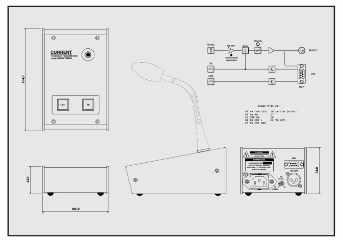
Talkback box Power supply built-in, all-in-one TB and CUE Built-in or goose neck
