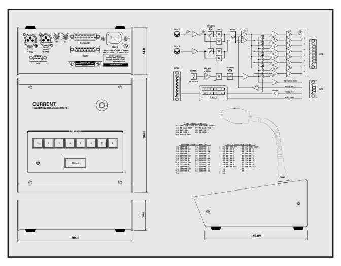
Multi talkback box 8 channel output All-in-one of the power supply built-in TB mix from ext The external control is possible Goose neck microphone
